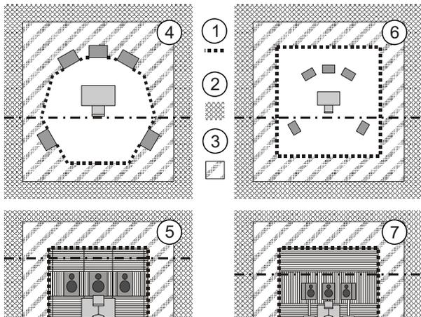
Fig. 1. – Some possible ways of MyRoom design: 1. air-transparent diffuse surface, 2. stiff wall, 3. low frequency absorption, 4. horizontal cross-section of room with soffit monitors, 5. vertical c.s. of room with soffit monitors, 6. horizontal c.s. of room with free-standing monitors, 7. vertical c.s. of room with free-standing monitors.
