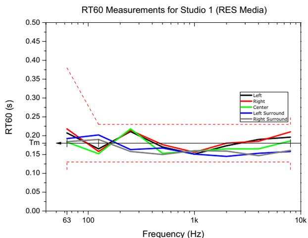
Fig. 3. -  $RT60$  Frequency dependence for the control room in the RES Media Studio, with AES limitations [9].
