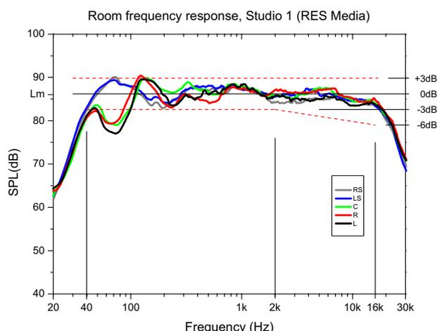
Fig. 5. – Acoustical frequency response of the surround control room in the RES Media Studio along with the limits defined in AES recommendations [9]. Graph shows the response of all five speakers.
