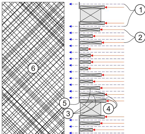
Fig. 2. – Side wall applied MyRoom treatment principle, horizontal cross-section, (top view): 1. air waves which passes through (blue/absorbed/diffused), 2. Air waves which cannot pass through (red/reflected/diffused), 3. Diffuser slats, 4. "Through hole" wells, 5. air transparent fabric, 6. Wideband absorber.
